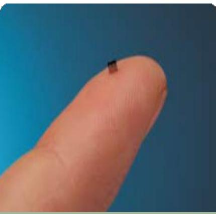
The Bluechiip® Cryogenic Delta Tag uses micro-electro-mechanical systems (MEMS), a relatively new technology that does not necessarily require electronic devices, transistors, capacitors etc., for operation. The tag communicates to the reader in the radio frequency spectrum but not the same way as typical RFID systems.
